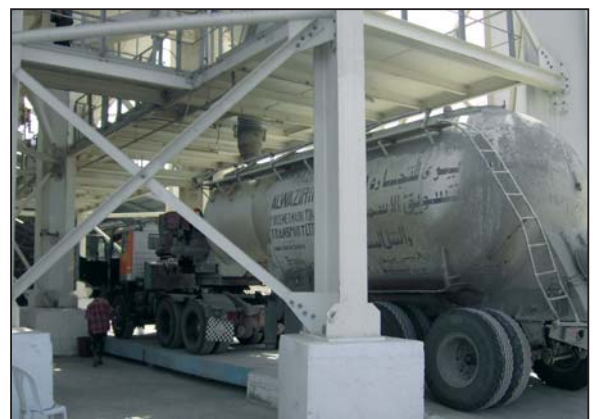
▲ Two silos equipped with jet loaders for bulk truck loading. All silos with safety equipments like overfill protections, level indicators, overpressure/vacuum flaps, dust filters and overflow pipes from silo to silo.
