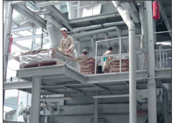
Front view of the Haver & Boecker ► packing machine with platform for empty bags.
